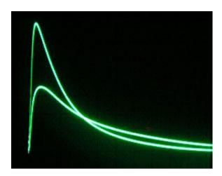
Figure 9 below shows both waveforms superimposed after the red binding post lead is reconnected and the Outer potentiometer is rotated clockwise to reduce the amplitude of channel 2 until it matches channel 1.
