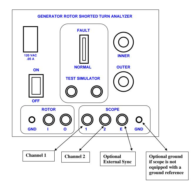
**3**. Power-up the instrument and the oscilloscope.
