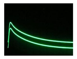
Figure 8 below shows both traces after the red binding post lead is disconnected and the Inner potentiometer is rotated clockwise to reduce the channel 1 amplitude by approximately one half.
