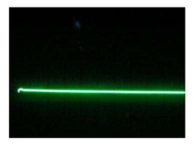
Figure 3 below shows an actual winding trace indicating the presence of one or more shorted-turns:
